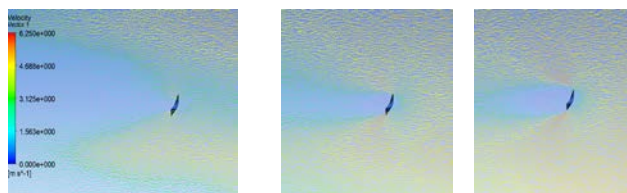
Figure 9 – velocity vector plots at (a) 0.02m, (b) 0.04m, and (c) 0.06m from the axis of rotation.
